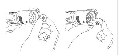
Fix the projection pattern in place by screwing the retaining ring with the provided PTTOOL.
