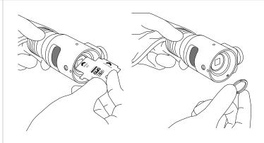
Remove the retaining ring using the provided PTTOOL instrument.
