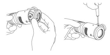
Insert back in place the C-mount adaptor and fix it by tightening the socket head set-screws with an M1.5 Allen key
