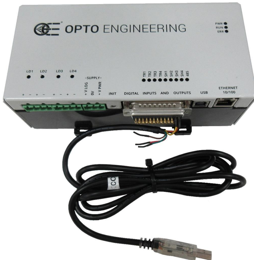
Figure 28: connection of RS485-USB adapter to the controller
