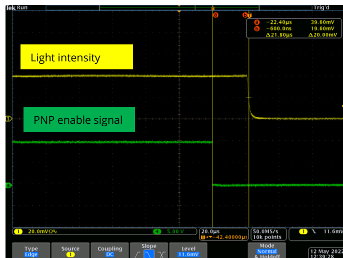
Figure 6: turn-off behavior for LTBRZ3-C series.
