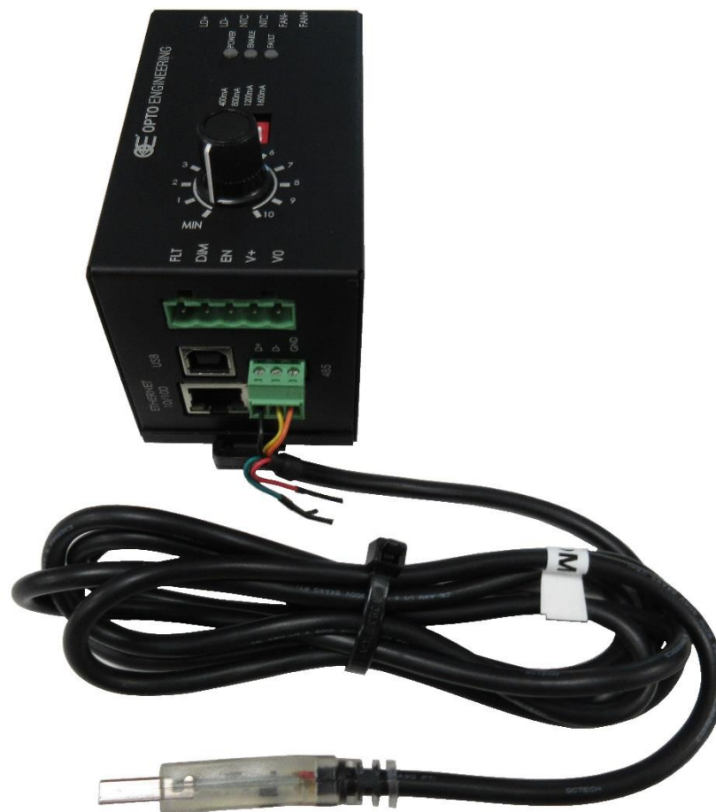
Figure 23: connection of RS485-USB adapter to the controller
